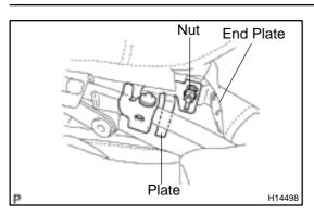
(h) By making the tarpaulin assembly in a full–open condition, remove the nut and end plate.
