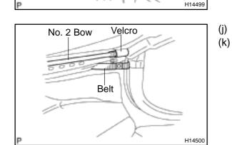
Remove the tarpaulin belt wrapped around the link side.Remove the velcro holding both ends of No. 2 Bow.
