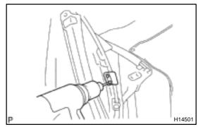
(o) Using a rivet cutter and a drill, drill out the rivets and remove the band.
